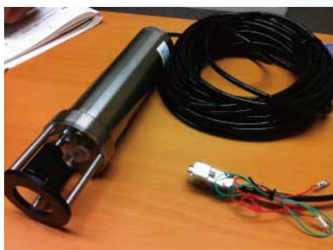
ACTW digital output version with D-sub connector
